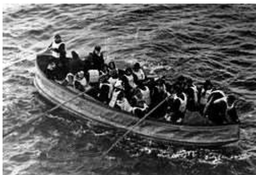
A collapsible lifeboat with canvas sides
