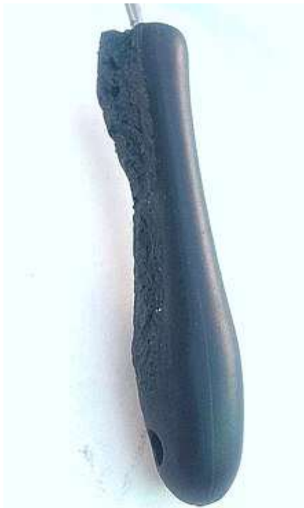
The plastic handle of a spatula that has been deformed by heat.
